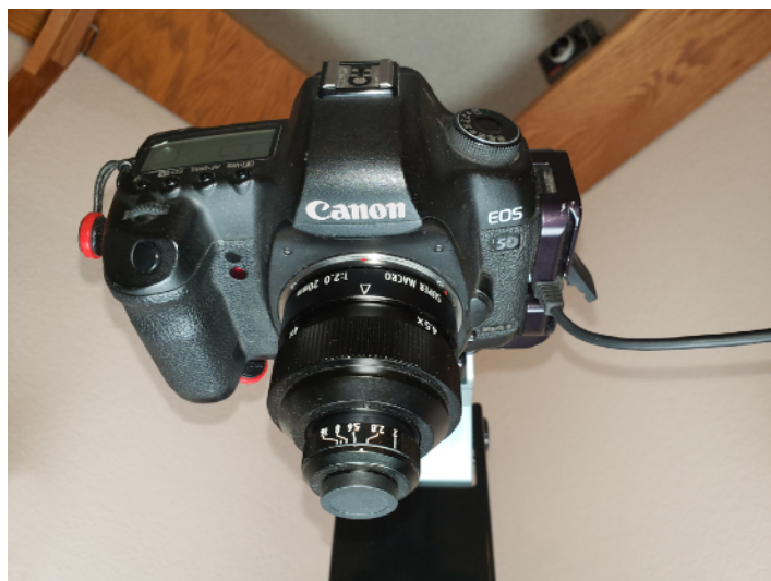
Figure 8. Mitakon 20mm f2 4.5X Super Macro mounted on a Canon EOS 5D Mark II.
