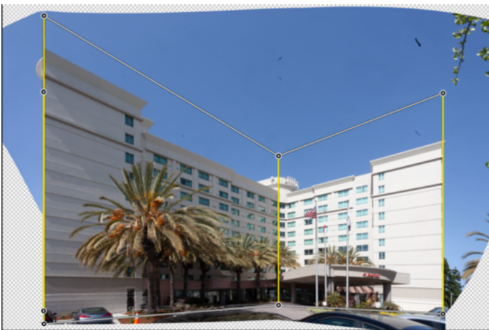
Figure 9. Perspective Warp in Warp Mode with shift-click used to make vertical corrections only. Shift-click turns the lines from white to yellow.
